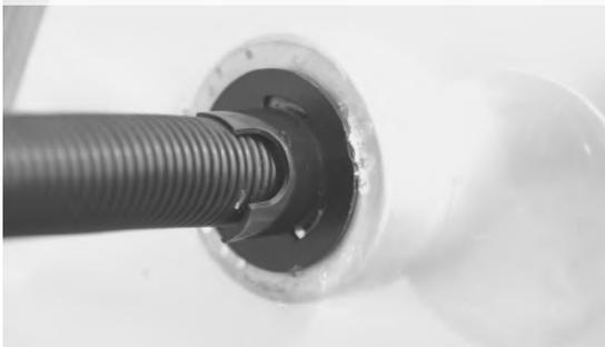
7- Insert hose into opening of fan and
